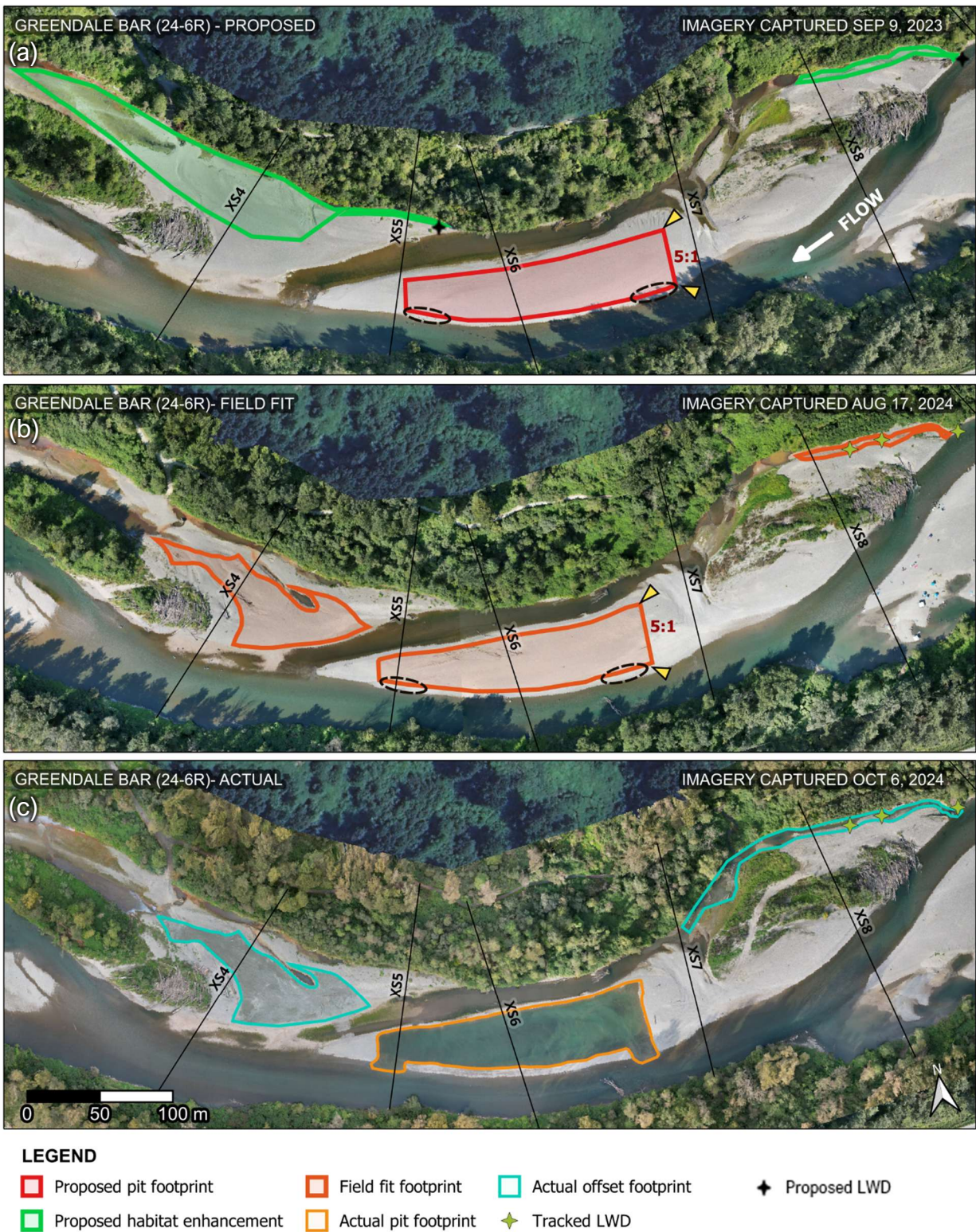
Figure 38. Orthomaps of Greendale Bar with (a) planned excavation and offsets based on 2023 river conditions, (b) field fit excavation and offsets based on current river conditions on Aug 17, 2024, and (c) actual excavation and offsets completed in 2024.
