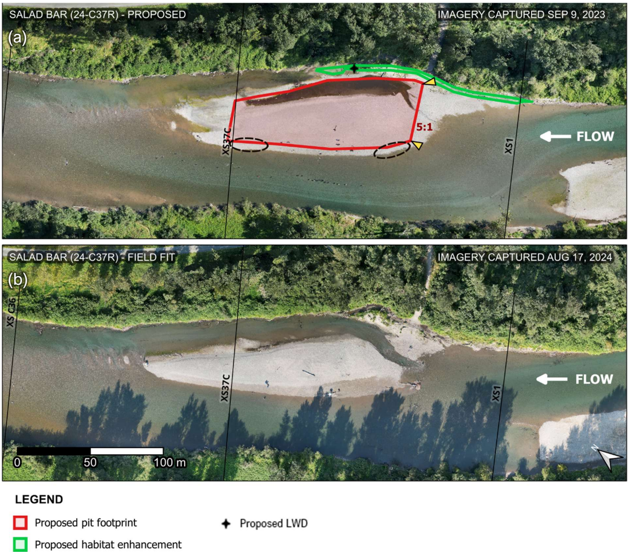
Figure 41. Orthomaps of Salad Bar with (a) the planned excavation and offset based on 2023 river conditions, and (b) river conditions on Aug 17, 2024.
