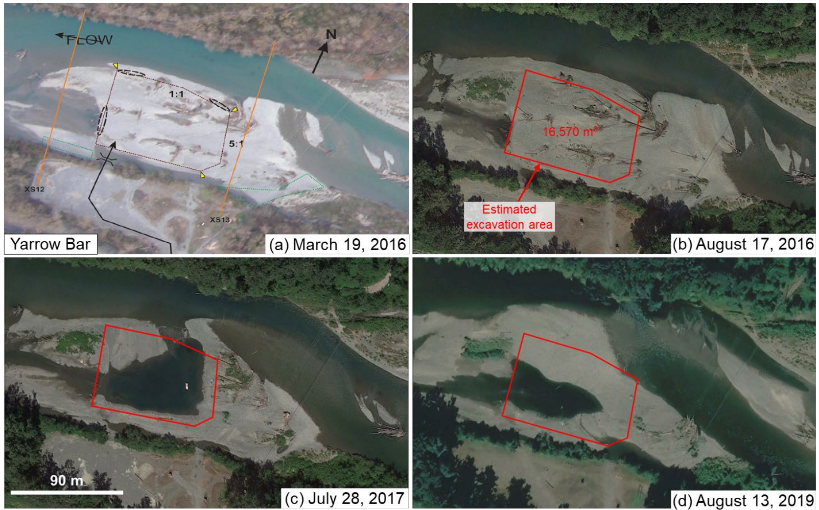
Figure A.5 Yarrow Bar on (a) March 19, 2016, (b) August 17, 2016, (c) July 28, 2017, and (d) August 13, 2019. Aerial imagery in (a) is from Nova Pacific (2016) while satellite images in (b) to (d) are from Google Earth. Sediment removal here occurred between August 27 and September 8, 2016. The image in (b) is before the sediment removal.
