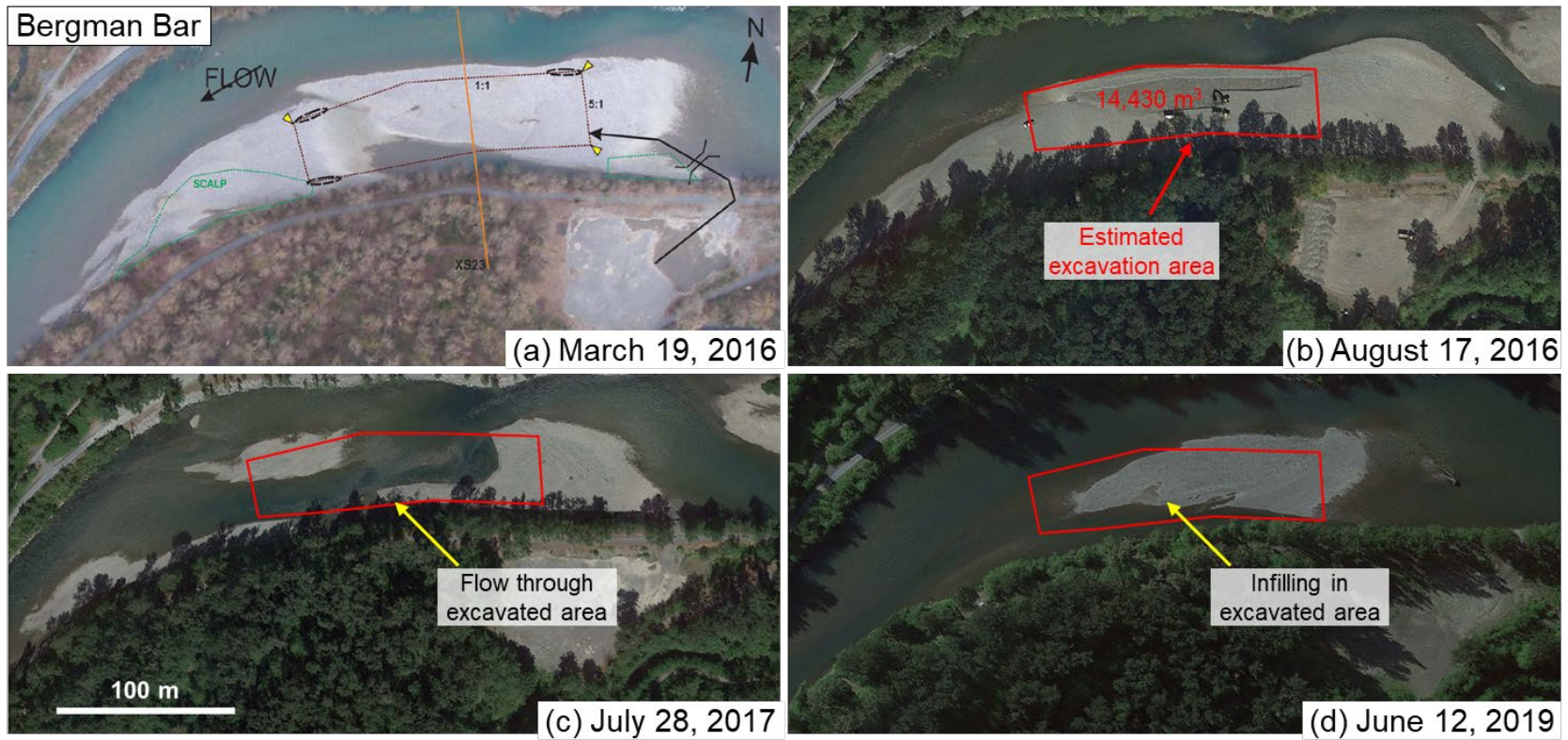
Figure A.3 Bergman Bar on (a) March 19, 2016, (b) August 17, 2016, (c) July 28, 2017, and (d) June 12, 2019. Aerial imagery in (a) is from Nova Pacific (2016) while satellite images in (b) to (d) are from Google Earth. Sediment removal here occurred between August 17 and August 26, 2016. The image in (b) occurred during the sediment removal.
