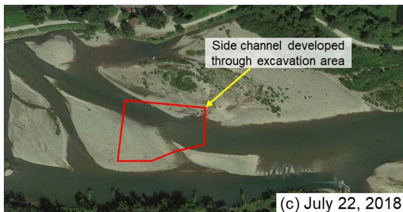
Figure A.2 Lickman Bar on (a) March 19, 2016, (b) July 28, 2017, (c) July 22, 2018, and (d) June 12, 2019. Aerial imagery in (a) is from Nova Pacific (2016) while satellite images in (b) to (d) are from Google Earth. Sediment removal here occurred between September 9 and September 27, 2016. There is no imagery available directly following the removal
