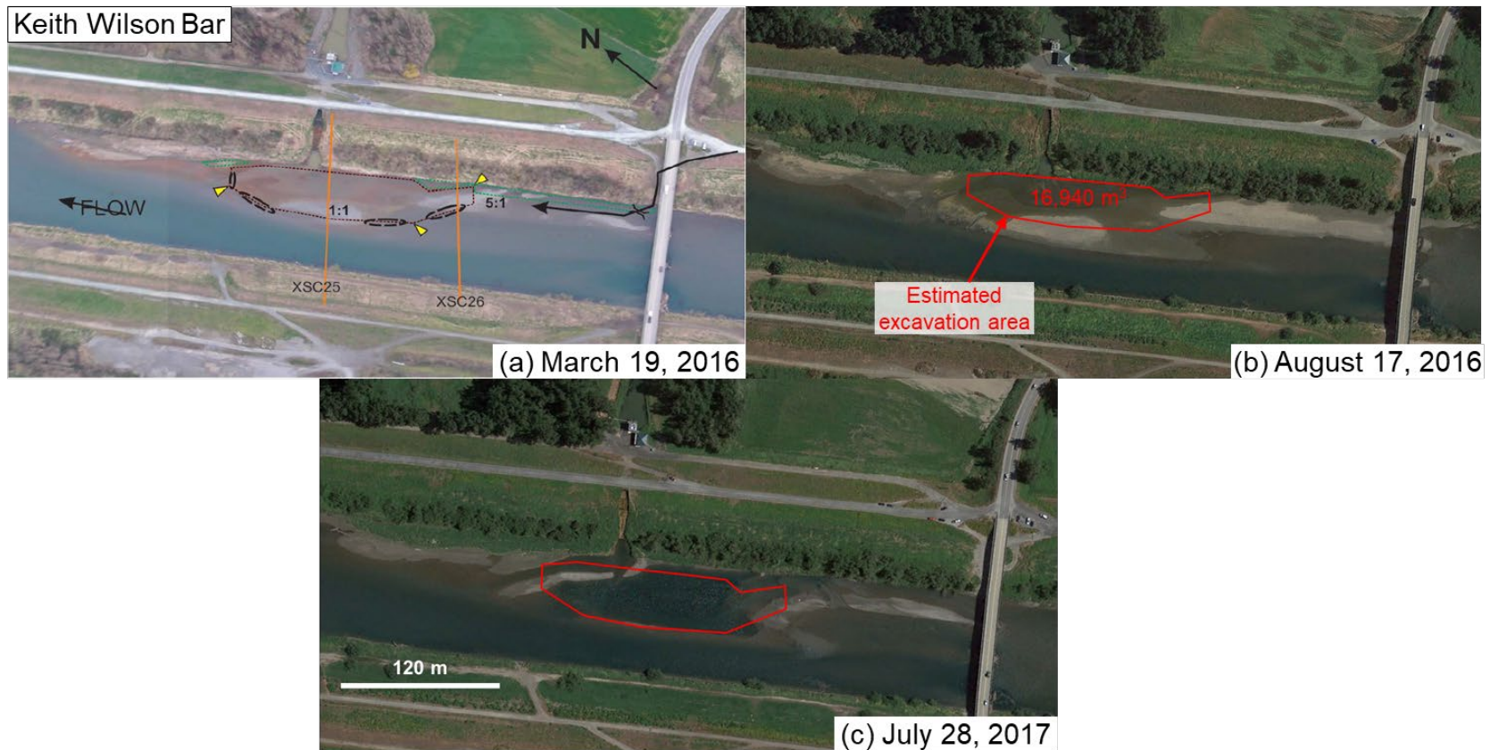
Figure A.6 Keith Wilson Bar on (a) March 19, 2016, (b) August 17, 2016, and (c) July 28, 2017. Aerial imagery in (a) is from Nova Pacific (2016) while satellite images in (b) and (c) are from Google Earth. Sediment removal here occurred between September 6 and September 29, 2016. The image in (b) occurred before the sediment removal. There is no imagery of the exposed bar in the years following 2017 due to high water levels.
