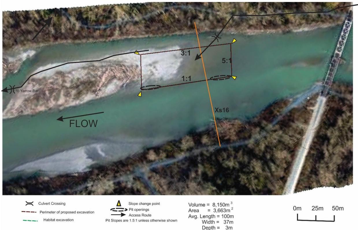
**Figure 9:** Railway D/S Bar excavation.
