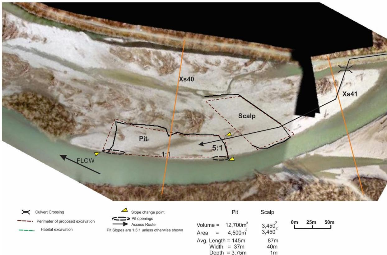
**Figure 9:** Peach Road D/S Bar excavation and scalp.
